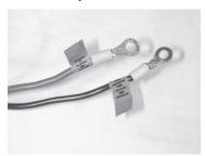
8. Route the red and black Remote Control-to-Battery cables from the Switch on the cable of the remote control, to the battery fuse box terminal strip in the vehicle. **The circuit fuse must be 70 amps.**
